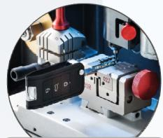
5. Cut the key blade and fix it in the Remote Car Key using the pins provided\*. SRP tells you what FH key blade to use.
