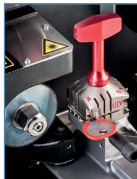
Flat and cruciform key cutting station
