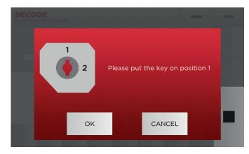
3. Put the key on position 1 and press **OK**. The machine will decode the first side of the key
