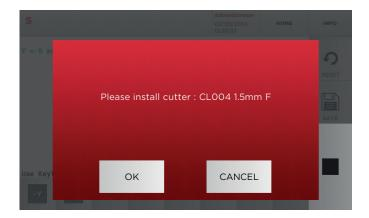
12. Install the required cutter (CL004 1.5 mm for edge-cut keys) and press **OK**
