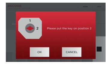
4. Put the key on position 2 and press **OK**. The machine will decode the second side of the key
