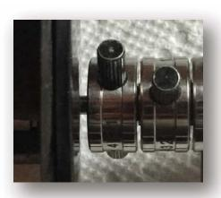
THE PICTURE ABOVE SHOWS THE PICK/READER FULLY INSERTED INTO AN 8 CUT DOOR LOCK. THE PICTURE BELOW SHOWS THE PICK/READER PULLED OUT 2 SPACES SO THAT YOUR MARK IS AT THE FACE OF THE LOCK. THE TOOL NOW READS SPACES 1-6. READ SPACES 3-8 FIRST, THEN PULL THE TOOL OUT TO YOUR MARK AND THEN READ 1-6 TO GET THE COMPLETE CUTS.
