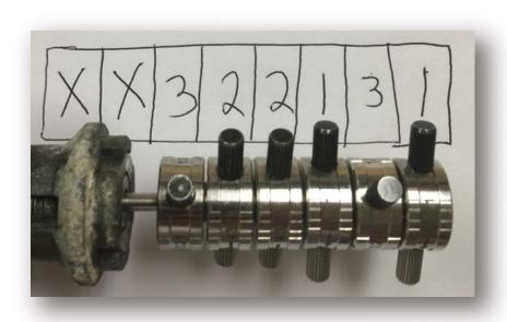
AFTER MODIFYING THE TIP OF YOUR TOOL YOU CAN NOW PICK 6 CUT TRUNK AND GLOVE BOX LOCKS, YOU CAN ALSO READ 8 CUT JAGUAR LOCKS – INCLUDING TRUNK LOCKS (SOMETHING THE 8 CUT READER APPEARS UNABLE TO DO SINCE IT HAS THE VALET TIP). THE CUTS FOR THIS LOCK ARE 21322131 YOU WILL NOTICE THE TOOL WILL DIRECT READ SPACES 3-8. SIMPLY ROTATE THE WHEELS IN THE UNLOCK DIRECTION, NO PICKING IS REQUIRED. SINCE THERE ARE ONLY 3 DEPTHS AND ALL WILL BE PRESENT DECODING IS QUITE SIMPLE TO DO.
