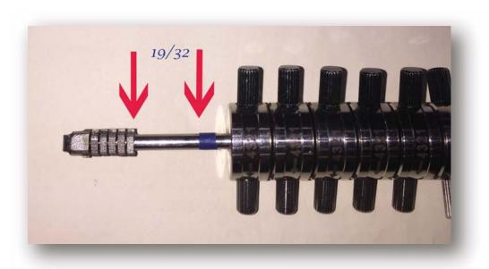
SO WHAT ABOUT CUTS 1 & 2? IN ORDER TO READ THESE SPACES WE AGAIN NEED A SLIGHT MODIFICATION TO THE TOOL. MEASURE BACK FROM THE REAR OF THE LAST TIP PIECE 19/32 OF AN INCH. SCRATCH A LINE ON THE NECK OF YOUR TOOL HERE. I'VE USED SOME BLUE PAINTERS TAPE IN THESE PICTURES FOR VISABILITY. WE WILL USE THIS MARK AS A GUIDE.
